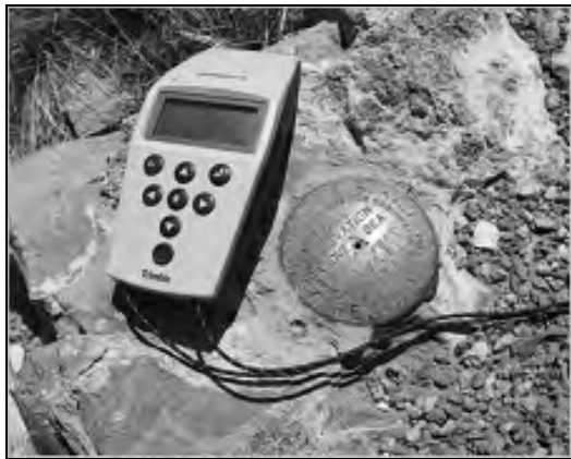
Figure 12. Trimble GPS system and survey markers.
